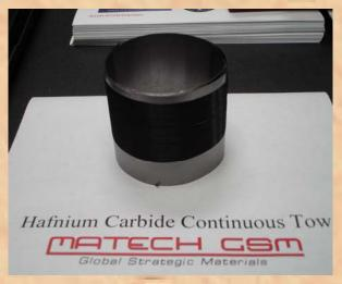
Dense, Nanocrystalline Fiber Continuous Tow Up to Multi-Hundred Filaments
